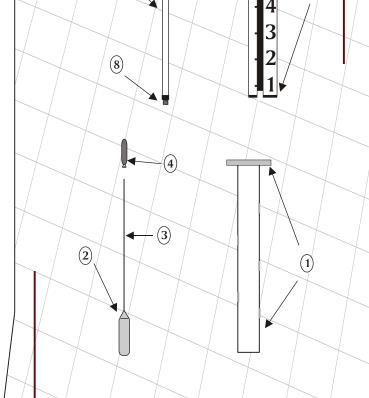
Approximate Floating Level - 20ft Rod SG of 1 = 8" (2 3/8" OD Float) / 4" (3.5" OD Float) SG of .9 = 9" (2 3/8" OD Float) / 4.5" (3.5" OD Float) SG of .8 = 10" (2 3/8" OD Float) / 5" (3.5" OD Float) SG of .7 = 11.5" (2 3/8" OD Float) / 6" (3.5" OD Float) SG of .6 = 13" (2 3/8" OD Float) / 7" (3.5" OD Float)
